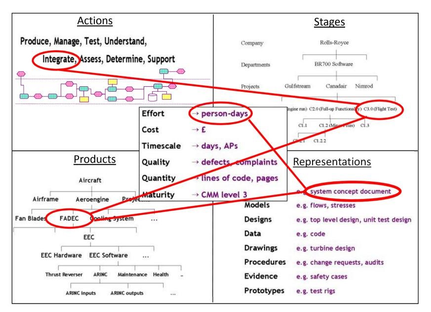
Engineer records: "I took 4 hours to Integrate Delivery C3.0 FADEC System Concept Doc Manager asks: "What was the total effort used to Produce the FADEC?"
